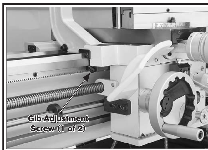
Figure 126. Front saddle gib adjustment screw.
